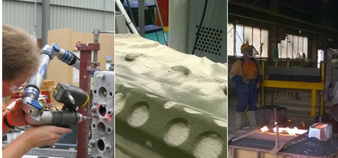
PHOTO: The original engine block is scanned, a 3D-printed sand mould is created, and the new engine block is cast. (Supplied: Philip Guilfoyle)
